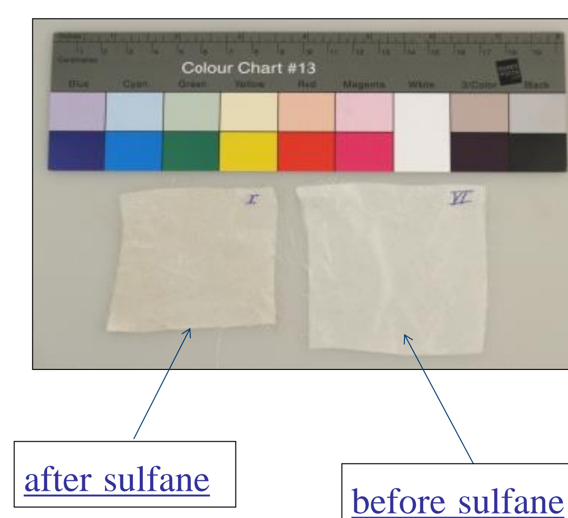
Fig. 7: The most significant colour change after sulfane treatment
