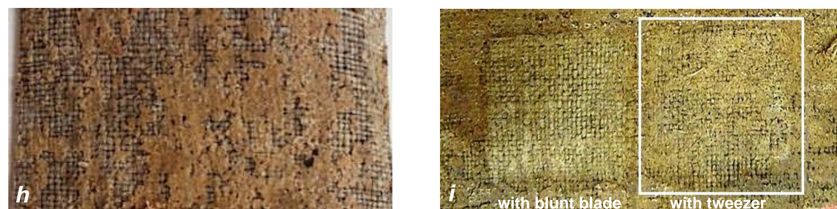
Detail of the lining canvas with glue before tests (h)
