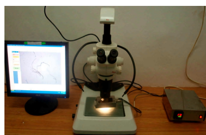
Fig. 1 MHT equipment comprises of a stereomicroscope coupled with a camera and a Hot Table equipped with a Central Processor both from Caloris (Romania).
