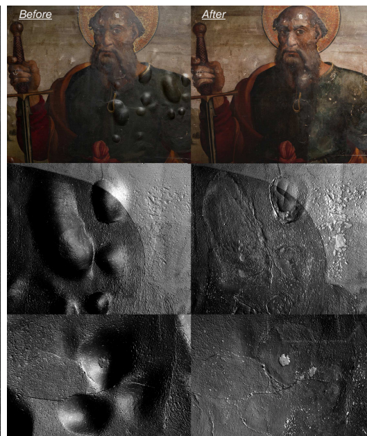
Fig. 3 Three details of a blistered paint layer, seen in RTI before (left column) and after (right column) planar correction. RTI provides better visualization of textural detail and brightness to make more objective comparisons and assessments of the effectiveness of the intervention processes.
